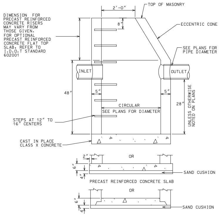
PREFABRICATED CONCRETE SLAB WHEN PRECAST REINFORCED CONCRETE SECTION ALTERNATE IS USED
